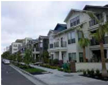
Building heights above the first two stories are encouraged to be stepped back to respect the heights of existing adjacent development.
