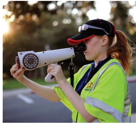
FIGURE 7: ELEMENT 7 NASAL RANGER FIELD OLFACTOMETER
