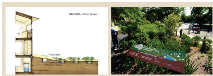
FIGURE: CLIVUS MULTRUM GREYWATER SYSTEM
