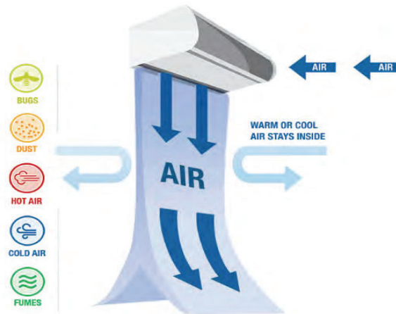
FIGURE 5: AIR CURTAIN OPERATIONS PROCESS
