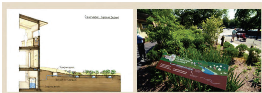
FIGURE: CLIVUS MULTRUM GREYWATER SYSTEM
