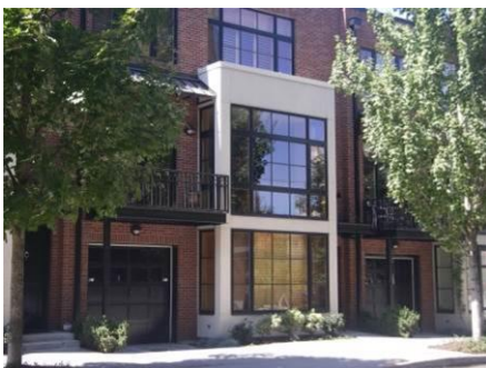
Building massing shall be broken to smaller massing, approximating the scale or form of existing adjacent structures.
