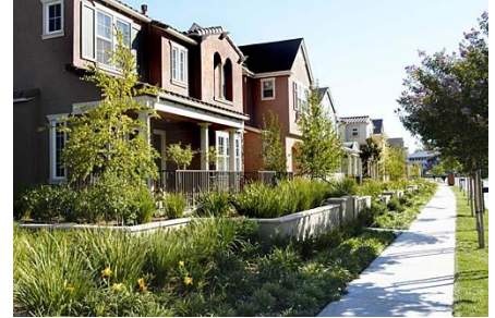
Front yard fences shall be set back, landscaped, and designed to be visually open above the first three feet.
